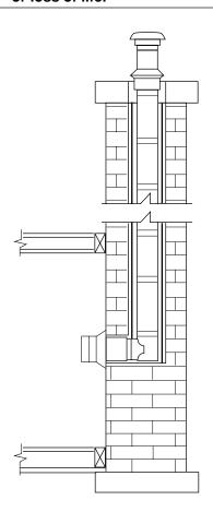
Figure 27 - Typical Straight Installation with Listed Chimney Liner
